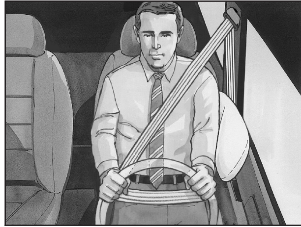
The seat-mounted side impact airbag for the driver is in the side of the driver's seatback closest to the door.
