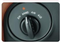
Envoy's four-wheel drive system rotary controls are located on the instrument panel.
